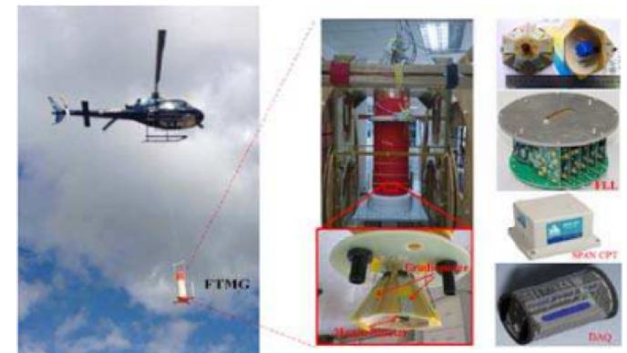
Figure1: schematic diagram of the airborne Superconducting FTMG system.
